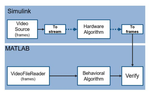
The MATLAB portion of this example loads the input video, runs the behavioral code, runs the Simulink model to import video frames and export modified video frames, and compares the MATLAB behavioral results with the Simulink output frames.
