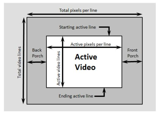
Create a visionhdl.FrameToPixels object and set the image properties. The image is an intensity image with a scalar value representing each pixel, therefore set NumComponents property to 1. This
